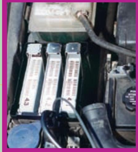
On this Volvo 850, transmission, engine management, and ABS computers are stored in an E-box in the engine compartment. Volvo previously stored the ECUs inside the passenger compartment area. The PCM monitors the ambient air temperature of this compartment via an NTC thermistor. The temperature value is available through serial data.
