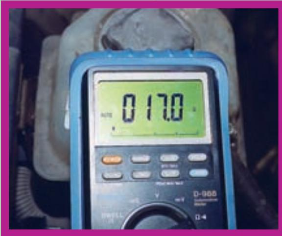
The injectors are high resistance type and should measure 17 ohms each. This eliminates the need for dropping resistors to control current flow. This is a sequential electronic fuel injection (SEFI) system, so each injector is controlled by a separate transistor inside the PCM. The system utilizes adaptive "self learning" to optimize fuel injector on-time under various running conditions.
