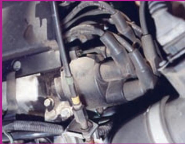
With the introduction of Motronic 4.3, the PCM now controls ignition timing directly. The need for a separate ignition computer has been eliminated. The power transistor mounted below the ignition coil is controlled by the Motronic PCM. The distributor shaft is driven by the camshaft and the rotor delivers spark to each spark plug. Two knock sensor inputs allow the PCM to selectively adjust ignition timing for any affected cylinder.
