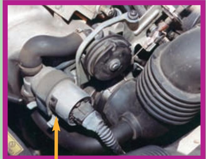
*Idle speed control is maintained by a standard Bosch idle valve. Ground signals from the PCM control the rotary vane opening angle and allow the PCM to control idle speed under all operating conditions. Two coil and single coil idle valve designs have been used on different Volvo models. Approximately 25-35 percent negative dwell represents a typical idle value.*
