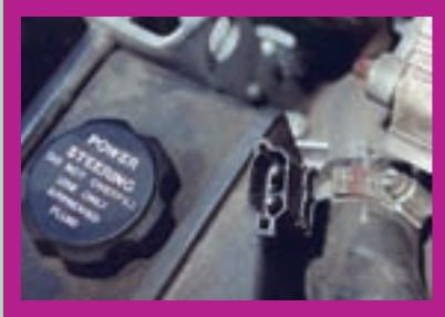
The coolant temperature sensor is mounted on the thermostat housing, just below the upper radiator hose. The sensor is not easily visible, but its resistance value can be checked by accessing the harness connector. This is a NTC-type sensor with a cold resistance of 2.4k ohms. Look for a resistance of approximately 300 ohms when the engine is at operating temperature.
